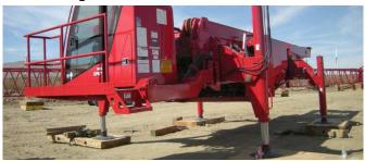
temporary roads to safely move equipment around on project sites. Mats distribute the weight loads from equipment and disperses it into the ground thus reducing the EPA or weight footprint of the equipment.
