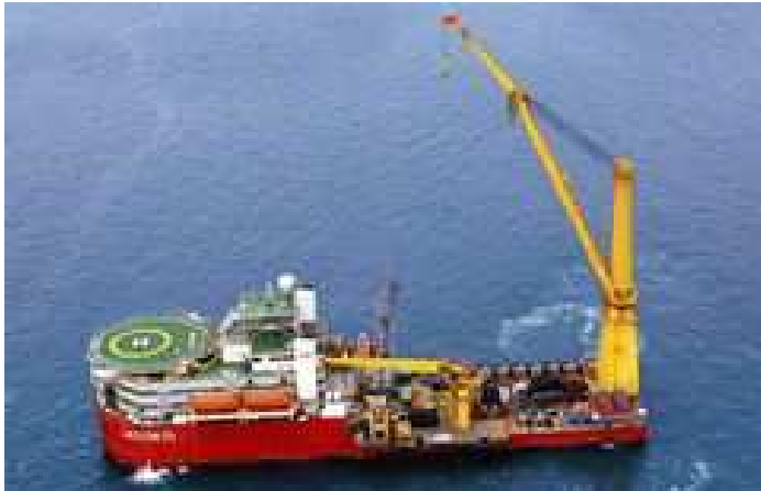
The Jascon 25 a pipe-lay construction crane vessel
