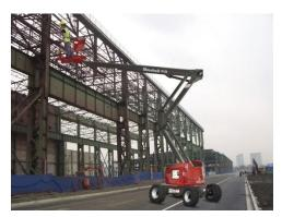
Mantall will feature its HZ160D self-propelled articulated boom with auto-leveling technology at this year's BICES exhibition in Beijing, China. The redesigned machine features a hollow chassis with a counterweight added to maintain stability, reducing the overall weight of the machine. It is well-suited to rough terrain with a maximum gradeability of 45%.
